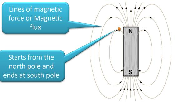
Lines of magnetic flux forms a closed loop
