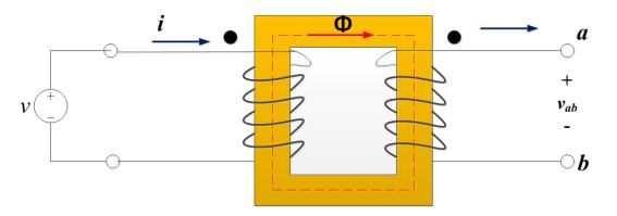
Let the coil on left side has  $N_1$  turns and inductance  $L_1$ , and the right side coil has  $N_2$  turns and inductance of  $L_2$ .
