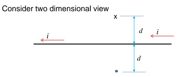
The magnitude of the flux density B at a point whose distance is d (measured perpendicularly) from the wire is given by
