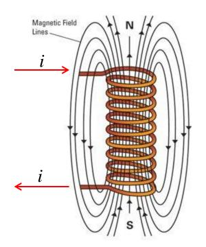
Right hand rule can be restated now *If the fingers on the right hand curl in the direction of the current then the thumb points in the direction of the magnetic field inside the core* This is cylindrical coil is also called as <u>Solenoid</u> If the radius of the core is *r*, and length of the cylinder is *l*, then, when *l*>>>*r*; Flux density of the interior of the core is approximated by
