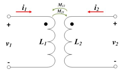
Connections may be from both windings, so  $i_1$  and  $i_2$  both are non-zero.
