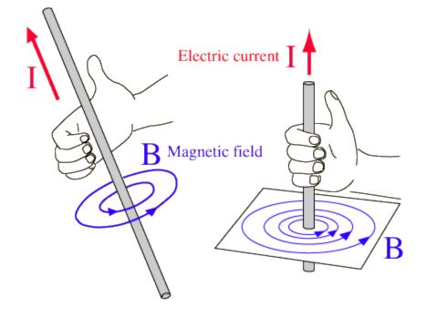
Consider a current I flowing through a long wire. Flux form a concentric circles around the conductor and the direction of the magnetic field is given by right hand rule.
