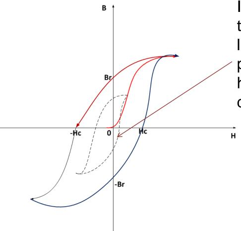
If the magnetic force applied to the demagnetized material is less than that required to produce saturation then the hysteresis loop is shown in the dashed line.
