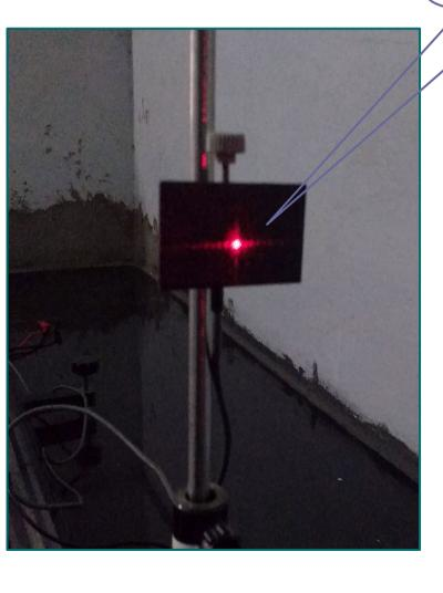
Diffraction from double slit
