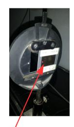
Slits to be used for diffraction
