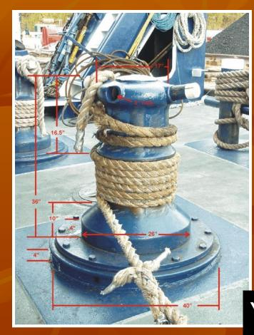
A rope is wrapped around a <u>fixed</u> drum, <u>usually for several turns.</u> A large load on one end is held with a <u>much smaller force</u> at the other where friction between drum and rope plays an important role
